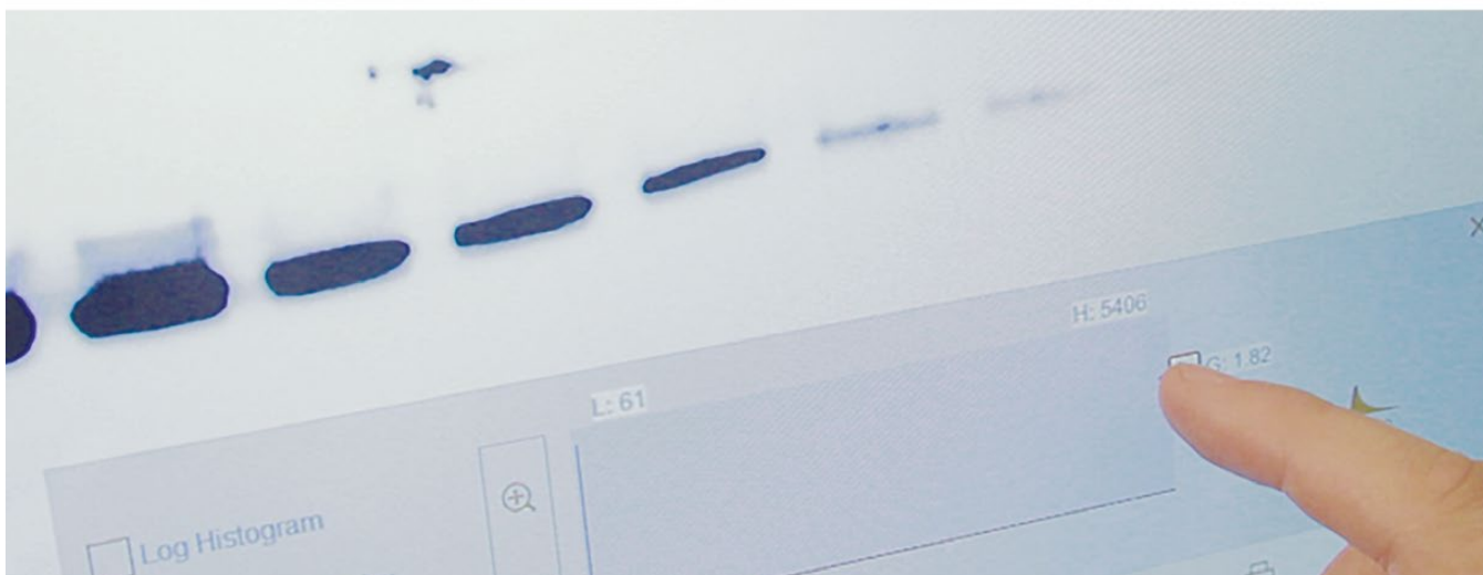
Researcher Ernesto Diaz-Flores loads a western blot membrane into the ChemiDoc Touch Imaging System using Smart Tray Technology™, which recognizes his imaging application, and then adjusts the camera and contrast settings automatically to obtain the optimal exposure for his protein of interest.
