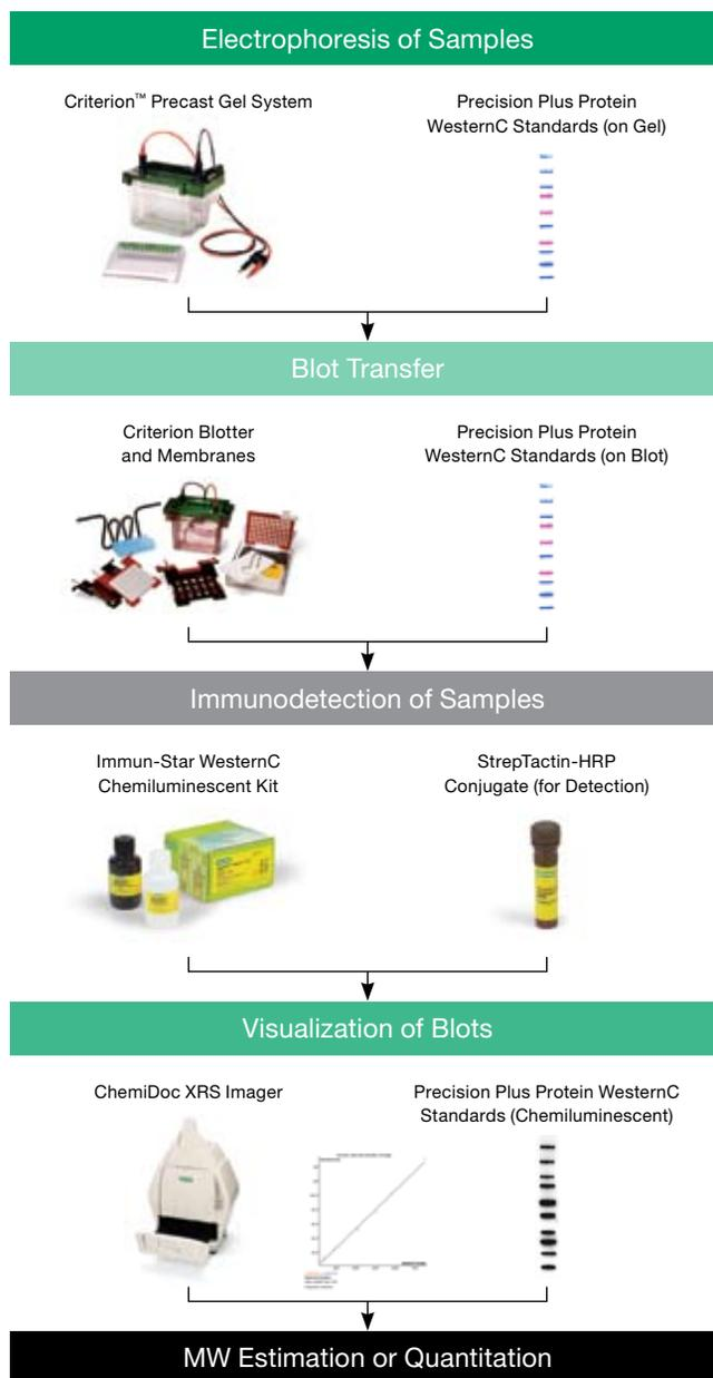
**Fig. 1. Western blotting workflow from SDS-PAGE to visualization and analysis.** The appearance of Precision Plus Protein WesternC standards at each step in generating a chemiluminescent western blot is shown on the right. Key equipment and reagents are shown on the left.
