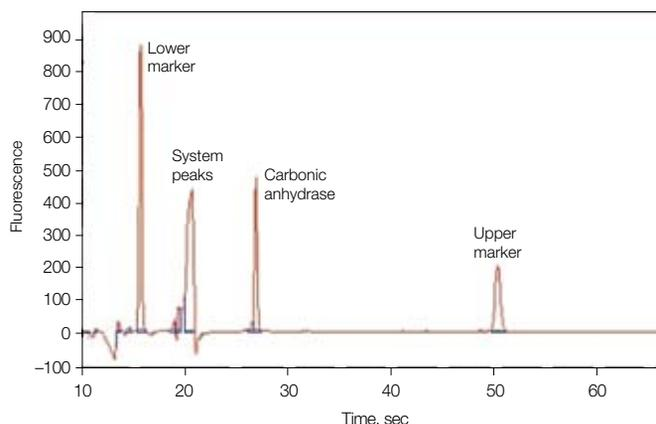
**Fig. 1. Experion electropherogram.** The positions of the upper marker (UM) and of a protein peak carbonic anhydrase are indicated. The UM is the default internal standard; however, carbonic anhydrase could be used as an internal standard.
