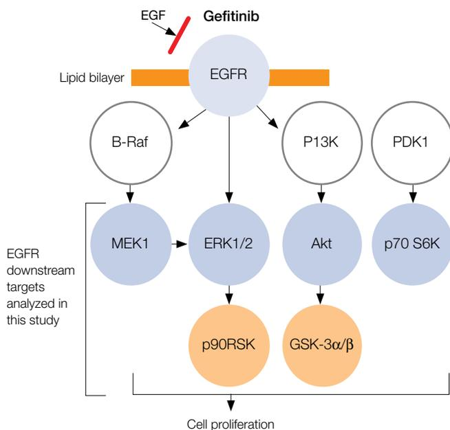
**Fig. 1. Schematic of the signal transduction pathway downstream of EGFR.** We used Bio-Plex phosphoprotein assays to detect the six phosphoprotein targets highlighted at bottom as well as p-EGFR. The drug gefitinib inhibits EGFR stimulation.
