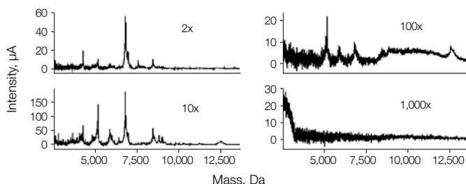
**Fig. 2. Optimization of sample concentration.** Different dilutions of lyophilized *Escherichia coli* lysate in binding buffer were spotted on a ProteinChip NP20 array. The numbers show the relative concentration of the sample compared to the original concentration (for example, a factor of 2x means 1/2 as much protein is present; the sample has been diluted 1:1). In this example, the 10x dilution shows the most peaks.
