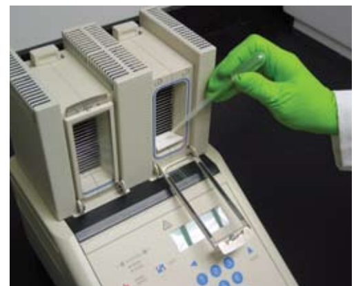
Fig. 3. Saturating the humidification pad with water.
