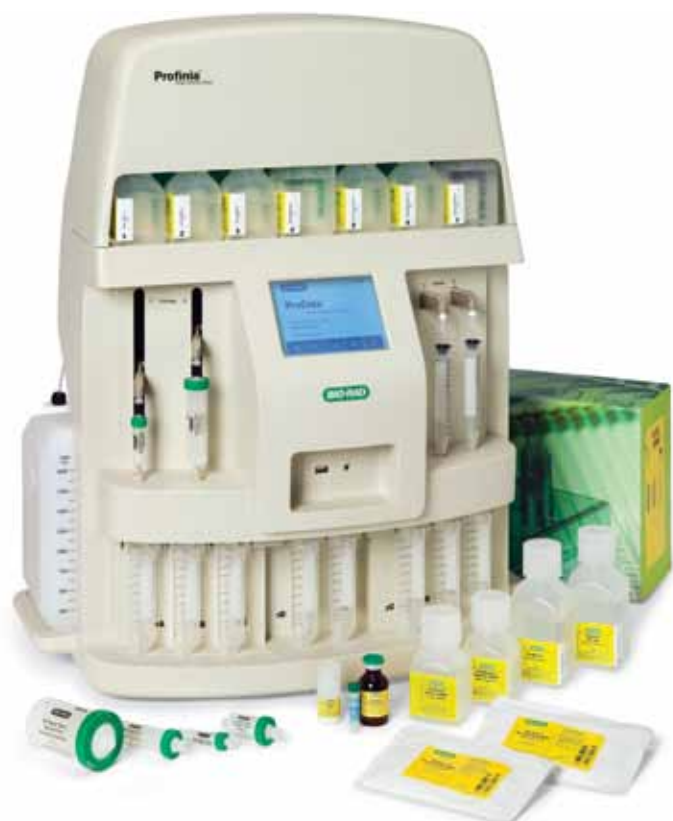
Fig. 1. Simple, automated, and reproducible affinity-tagged protein purification. The Profinia system works with prepackaged buffer and cartridge kits. The instrument features a small benchtop footprint (49 x 33 cm) and a space-saving, compartmental configuration that houses all reagents, sample and collection tubes, and cartridges on the instrument. A central compartment provides convenient storage for a touch-screen stylus and access to a USB drive for run data capture and export.
