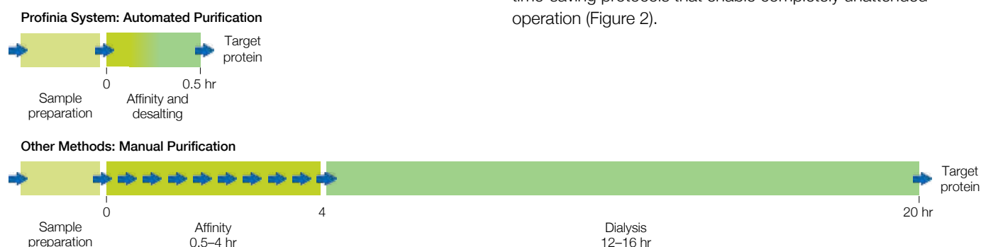
Fig. 2. Time and labor savings with the Profinia system over manual methods of affinity-tagged protein purification. Typical ranges in time required for purification of target proteins are shown. The Profinia system's self-contained hardware and preprogrammed software methods accelerate His- and GST-tagged protein purification. The system combines affinity purification with automated desalting, compared to separate processes for affinity and desalting in the manual methods. ➡, hands-on step.
