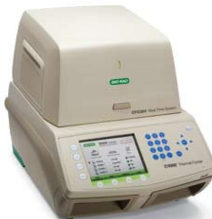
The CFX384 system maximizes fluorescence detection for specific dyes in specific channels — the optics shuttle individually illuminates and detects fluorescence from each well with high sensitivity and no cross talk. At every position and with every scan, the optics shuttle is reproducibly centered above each well, so the light path is always optimal and there is no need to sacrifice data collection in one of the channels to normalize to a passive reference.
